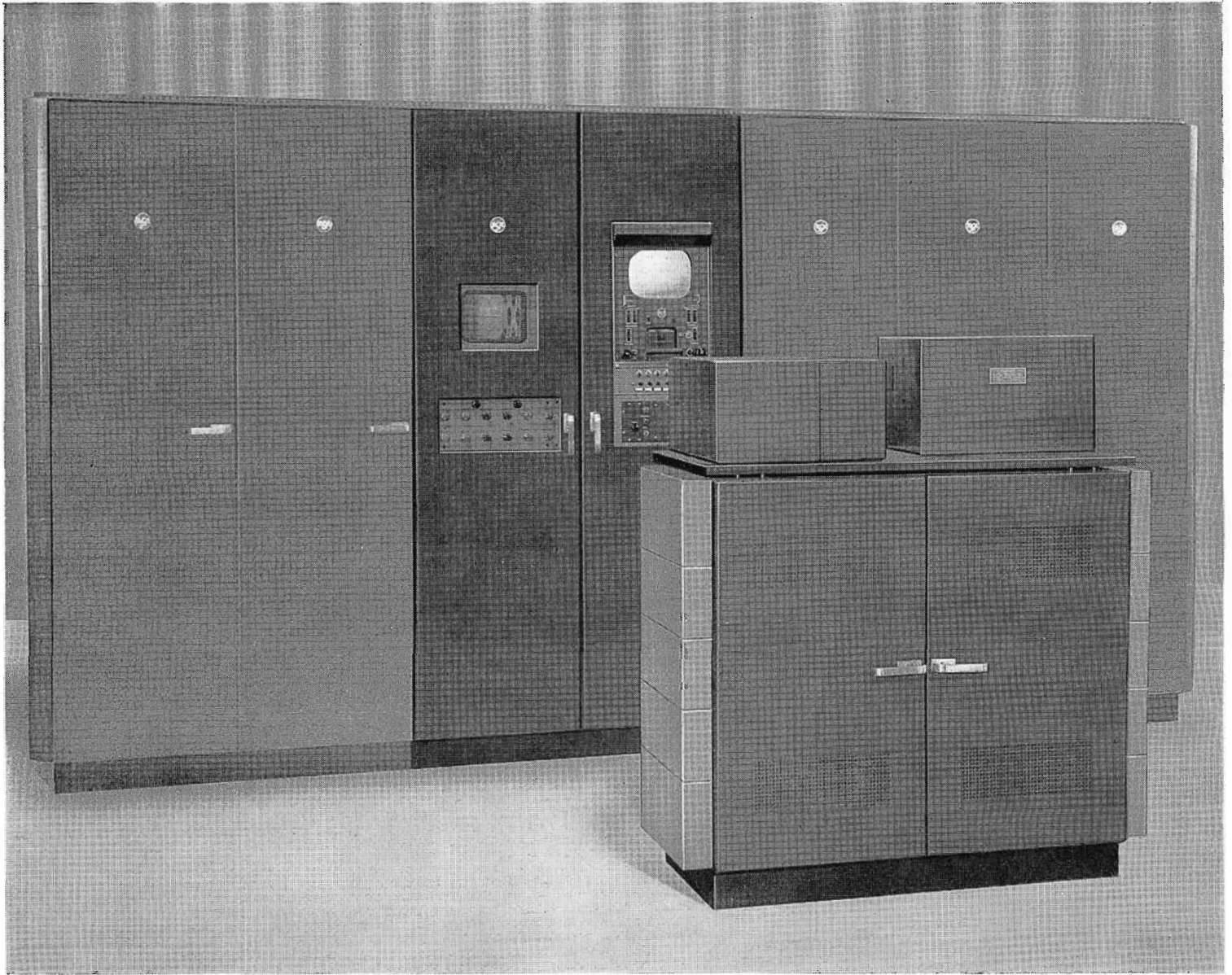
FIG. 1. The above system, with the Color Slide Camera shown in the foreground, has been supplied to laboratories for color receiver testing. The third tall rack from the left contains a three-Kinescope monitor. To the right of this cabinet is a rack-mounted master monitor, push button panel and Color Slide Camera Remote Control Panel. Adjacent racks house the sync generator equipment, gamma amplifier, colorplexer, decoder and power supplies. For broadcast service, these racks of equipment (less the three-tube monitor and the rack-mounted master monitor) are supplied as accessories.
